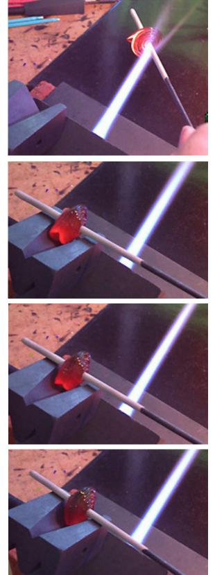
After the two sides connect, evenly heat the entire bead. You can actually see it puff up a bit as the heat expands the glass.
