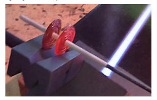
Roll the two warm disks into the groove so they kiss each other and connect. Then keep rolling.
