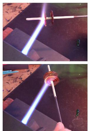
Position the Groovy Tool up near the torch with the largest groove on top.
