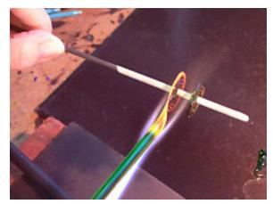
Build the disks simultaneously, alternating between the two disks as you build them. This keeps both disks warm and helps prevent cracking.
